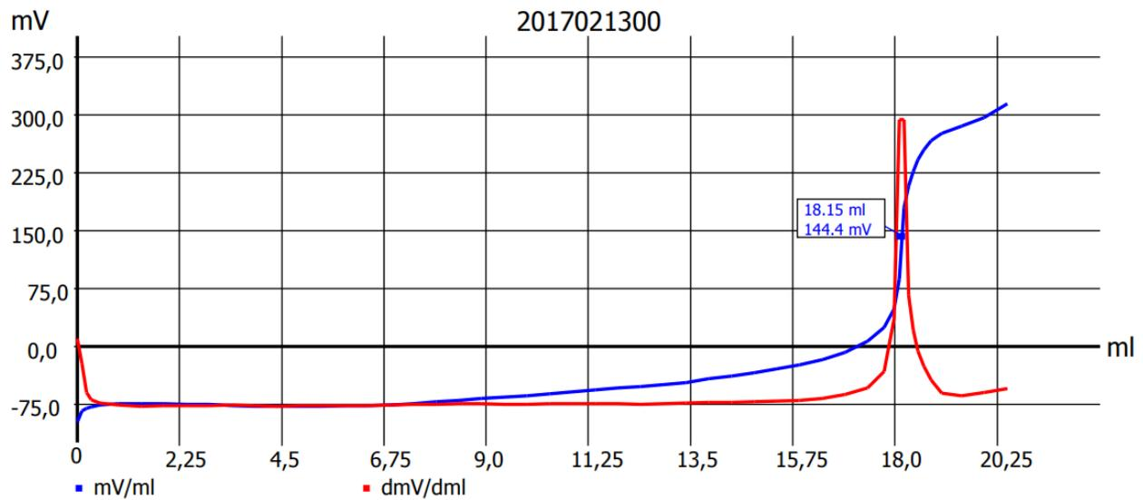
For the sample titration, the same parameters are used as for the blank determination.
